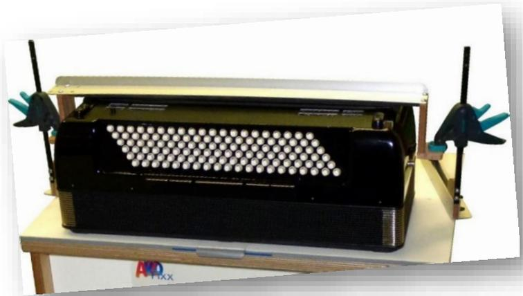
Reversing the wind direction from push to pull is done very quickly (5), so checking for any reed which sounds incorrectly is a piece of cake.
